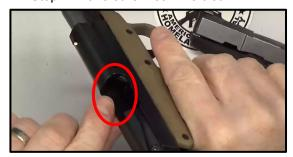
Step 3: Rack the slide and take flat tip screwdriver and remove the takedown pin
