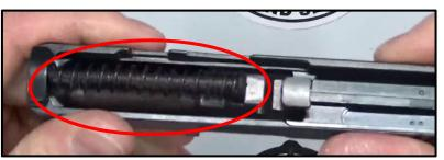
Step 6: Get your M\*CARBO Stainless steel Guide Rod and Recoil Spring, and place the guide rod in the spring
