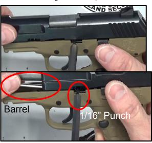
Step 10: Take your takedown pin and drop it right in, and make sure the ledge is on the bottom, and press on it until you hear it snap into place
